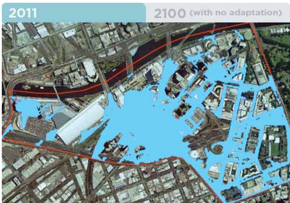
Areas of Southbank potentially flooded by up to 20 centimetres of water after a 1 in 100 year rainfall event in 2011.
