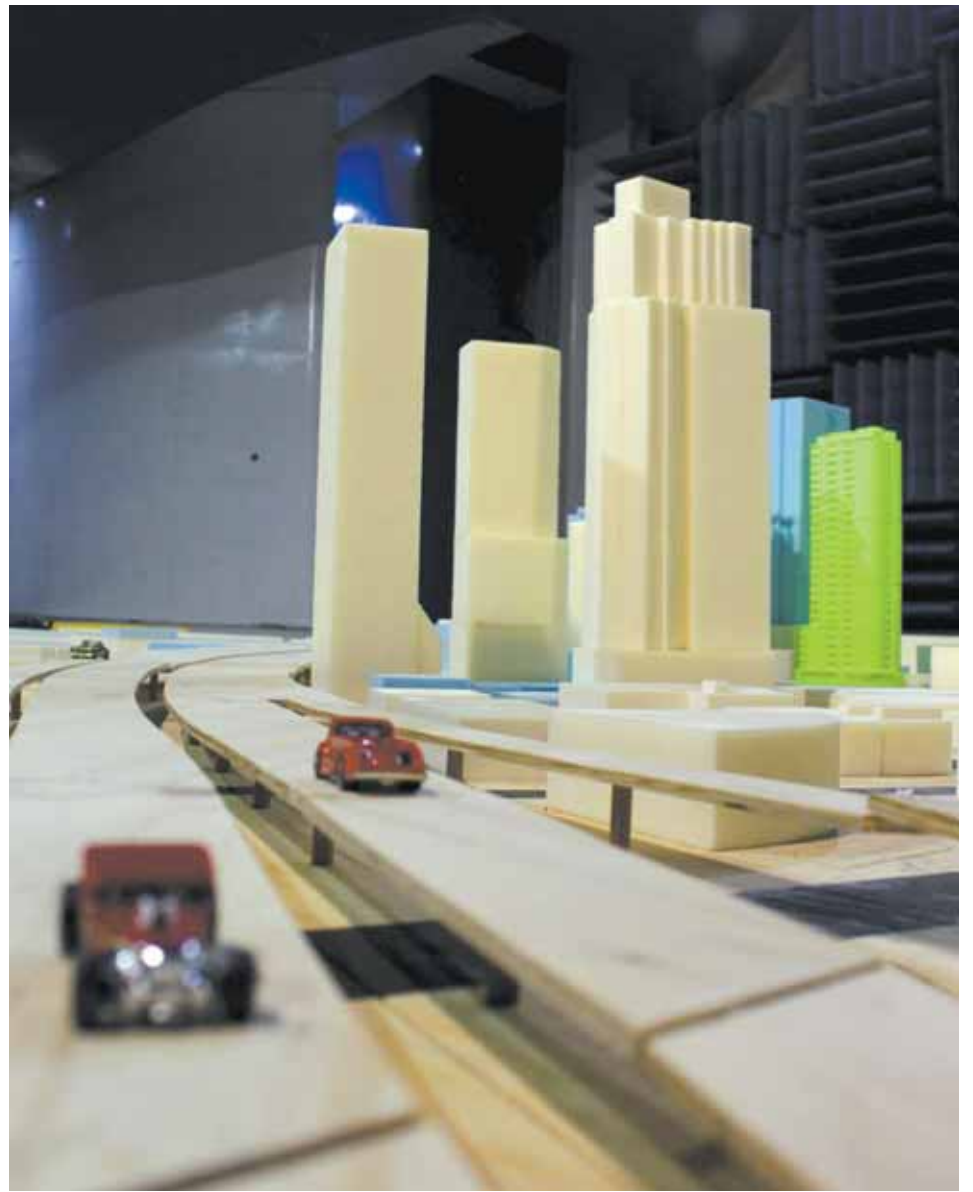
A recent wind tunnel test conducted at Monash University in Clayton for a Southbank development.
