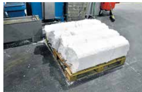
Air compressed polystyrene compacted into blocks.
